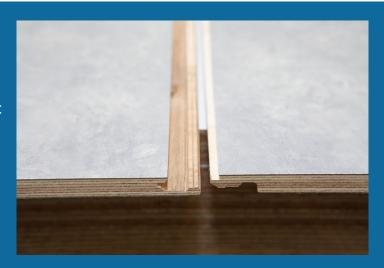
Continue with the same process as above, until the fitting of the last panel, finishing off with an end cap (removing the groove first to ensure extrusion is fitted neatly).
